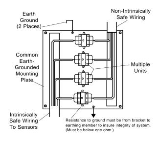
Note: All intrinsically safe wiring must be segregated from non-intrinsically safe wiring.
